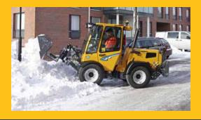
Wille 275 is agile and robust. Its minimum width is 1,260 mm and minimum height 1,990 mm. It has operating hydraulics with a flow of 110 lpm. Wille's extensive range of work attachments and tyres makes it a perfect partner.
