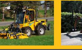
Inner turn radius 1890 mm Outer turn radius 3200 mm
